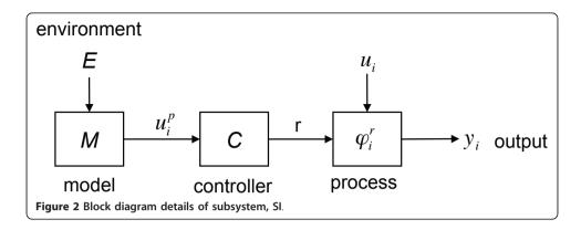
The input to the model, E, is from the environment. The model output, the predicted input for the process, is sent to the controller. The output from the controller, r, is the control vector and is sent to the process, as are other inputs from other subsystems. It is important to realize that the process,  $\varphi_i^r$  governs the subsystem,  $S_i$  which processes its input,  $u_i$  (t + h) at a later time t + h.
