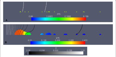
**Figure 8** An example of a QS biofilm under high nutrient conditions, EPS consumption case. The composition of the biofilm by EPS biomass is shown (A) before and (B) after induction. The carbon concentration scale is given in (C).
